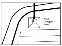
The antenna may be mounted along the top of the front or rear window. For best performance, don't mount on the rear window of trucks or SUVs.
