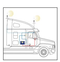
For best performance, it is important to install the antenna as high on the truck cab as possible. The radials should be no lower than the top of the truck cab. We recommend that when using a Wilson Electronics mobile wireless signal booster, to install the trucker antenna on the top, rear area of the cab, the grab bar or the headache rack.
