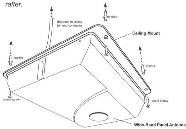
Drill a hole large enough to accommodate the dimension of the connector on the location you have marked for the cable. Hold the antenna to the ceiling and mark the locations for the screws and then
