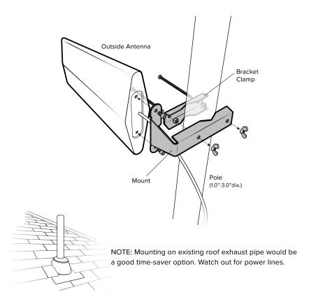
Point the **outside antenna** toward the nearest cell phone tower. To find the nearest tower, use an app such as 'Open Signal'. **This is the most critical step of the installation process because it will determine the overall performance of the booster's system.**
