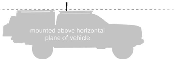
For best performance the outside antenna should be mounted above the horizontal plane of the vehicle and/or above other gear on top of the vehicle.
