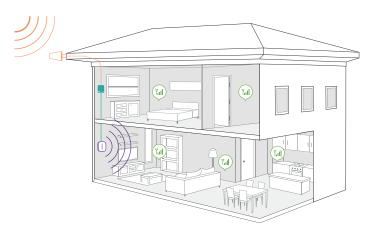
**Receives signal:** The outside antenna reaches out to access the existing strong outdoor cell signal and delivers it indoors to the booster.
