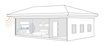
**Receives signal:** The powerful outside antenna reaches out to access a voice and 3G, 4G, and LTE data signal, and delivers it to the booster.
