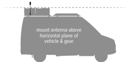
For best performance the outside antenna should be mounted above the horizontal plane of the vehicle and/or above other gear on top of the vehicle.
