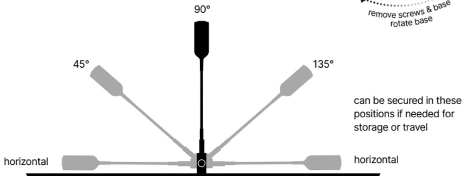
NOTE: System will only fully function with the antenna in the upright position.
