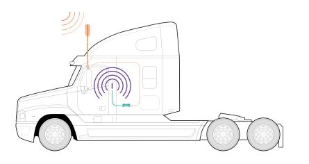
**Receives signal:** The powerful antenna reaches out to access voice and data signals, and deliver them to the booster.
