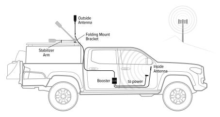
Use stability arm to secure antenna when laid in the horizontal position.
