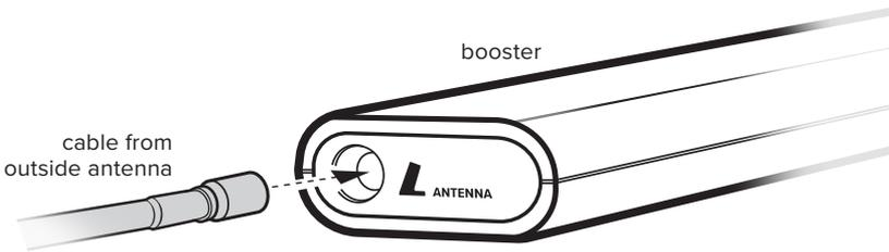
The included Velcro® can be used to mount the booster out-of-the way on the floor under a seat or mounted to the side of the trunk. It is best to mount in a place where the cables cannot be tripped over or snagged (damaging the booster).
