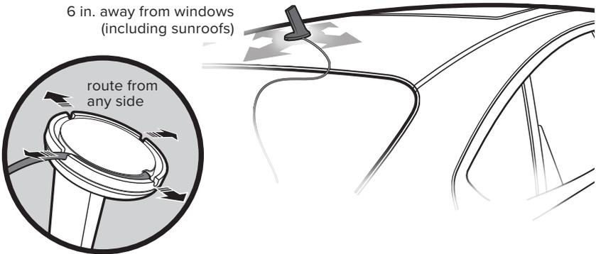
NOTE: For roofs that are non-magnetic, call Tech Support **866.294.1660**, for an adhesive disk to mount the outside antenna.
