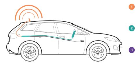
**Receives signal:** The powerful antenna reaches out to access a voice and 3G, 4G, and LTE data signal, and delivers it to the booster.
