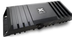
AC power is required if you want to use the CEL-FI GO G32 booster in its 100 dB *Stationary* mode for maximum inside coverage while you are parked. On DC power, the booster will only operate on 65 dB *Mobile* mode used while underway. (See sidebar.)
