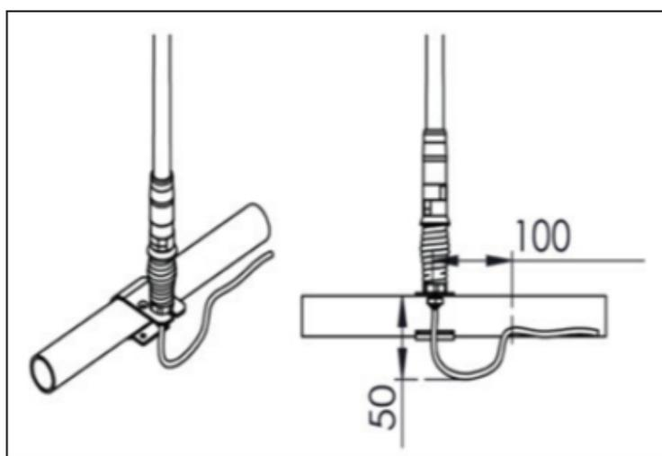
**Important:** When installing any spring-loaded antenna, it is important to allow enough loose cable at the base of the antenna for when the spring flexes. A loop of 50mm before fixing the cable would be sufficient for 8100 Series antennas (see pictures).
