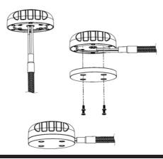
Magnetic surface for Optional Magnet Base kit installation
