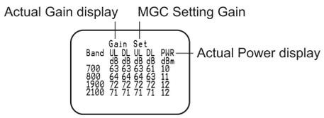
**Note:** When adjusting the gain manually, please ensure that the uplink gain is equal to or not 5 dB less than the downlink gain setting. This avoids interference with the local cell site tower network.
