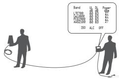
The outdoor antenna receives the strongest signal when the booster's downlink output power reaches its highest level in each band. If the LCD shows maximum gain and power, and there are not any alarms (no ISO, ALC, OFF legend flashing and no quick flashing green or red in LED), it means the present location is the best for ensuring that the booster has maximized performance. The maximum downlink power for F27-5S Telicos is 27dBm, and the maximum downlink gain is 83dB.
