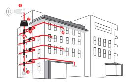
1.Outdoor Wide Band Directional Antenna 2. Booster 3. Indoor Wide Band Panel Antenna 4.Coupler 5. Splitter 6. Indoor Wide Band Dome Antenna
