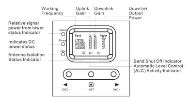
**Band:** Shows the working frequency bands where the booster is operating.
