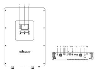
1.LCD 2.LED indicators 3. Control buttons 4. DC 12V 5. Outdoor antenna port 6. Alarm 7.Net 8.Run 9.BAT On/Off 10.Ethernet port 11. Local port 12. SIM Card 13.Antenna 14.Indoor antenna port 15. RS232
