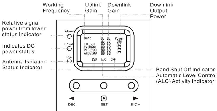
**Band:** Shows the working frequency bands where the booster is operating.
