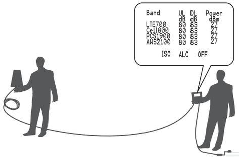
The outdoor antenna receives the strongest signal when the booster's downlink output power reaches its highest level in each band. If the LCD shows maximum gain and power, and there are not any alarms (no ISO, ALC, OFF legend flashing and no quick flashing green or red in LED), it means the present location is the best for ensuring that the booster has maximized performance.
