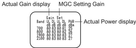
**Note:** When adjusting the gain manually, please ensure that the uplink gain is equal to or not 5 dB less than the downlink gain setting. This avoids interference with the local cell site tower network.
