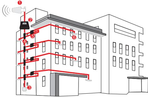
1. Outdoor Wide Band Directional Antenna 2. Booster 3. Indoor Wide Band Panel Antenna
