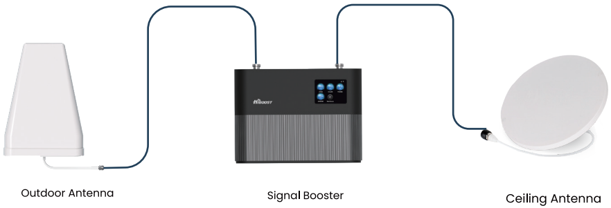
Figure 4 — Correct booster cable routing. Outdoor antenna to OUT; Indoor antenna to IN.
