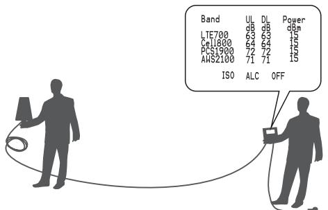
The outdoor antenna receives the strongest signal when the booster's downlink output power reaches its highest level in each band. If the LCD shows maximum
