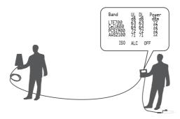
The outdoor antenna receives the strongest signal when the booster's downlink output power reaches its highest level in each band. If the LCD shows maximum
