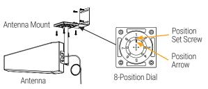
Optimize the donor signal by pointing the antenna properly. Use the Cel-Fi 8-position mount with a directional antenna, and the AntennaBoost feature on the WAVE app, to determine the optimum direction to point the antenna.
