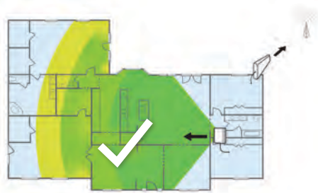
Face inside antenna away from outside antenna
